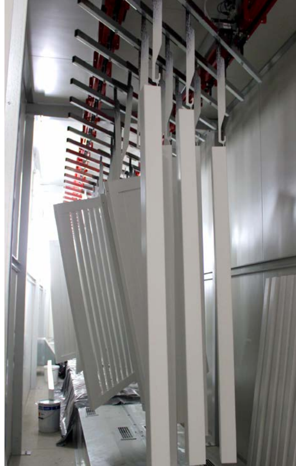
Painted products in drying chamber
