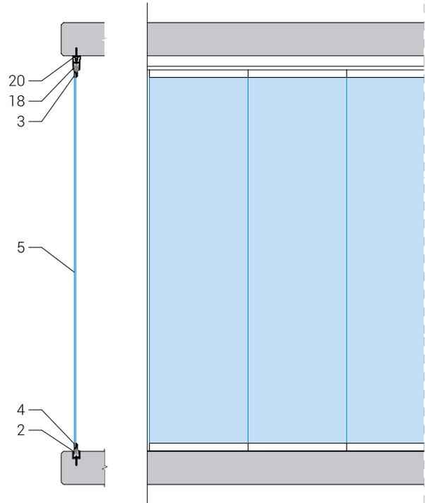
Lower fixing with U-steering profile
