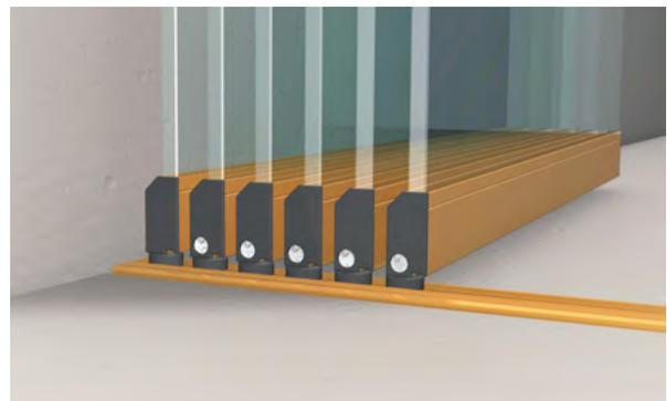
The structural integrity of the system is critical for the proper functioning of the unit. The deflection of the upper and lower steering profile under full load should be limited to a maximum of 2 mm per side.
