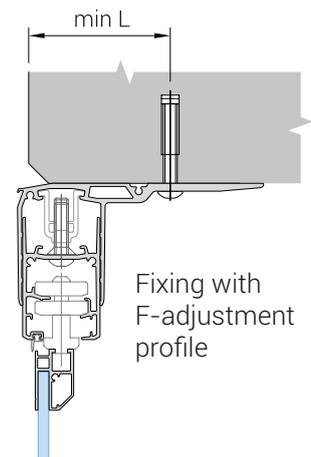
The extremes of the profile mounting holes are a minimum of 35 mm and a maximum of 55 mm from the right edge of the profile. A support surface must be provided from the centre of the mounting hole to the right end of the profile.
