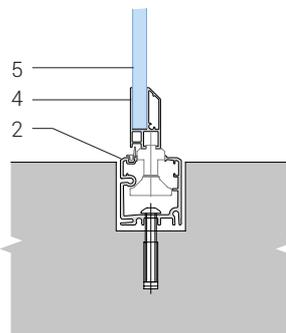
Upper fixing with U-adjustment profile
