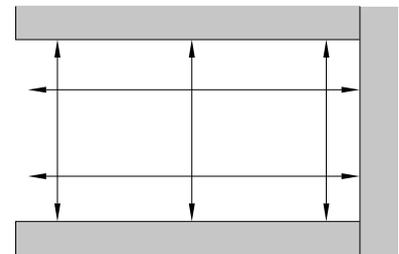
1. **Glasses parallel to the lower edge:** Height measure = Opening measure + 90 mm - reductions
