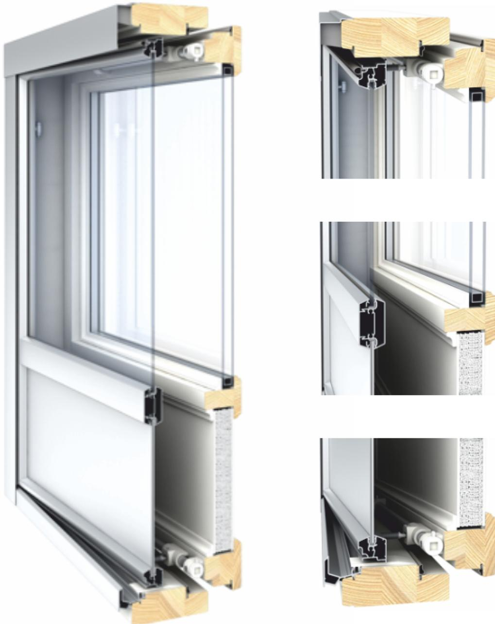
**Fenestra French** is a twin leaf wood-aluminium balcony door with an aluminium clad frame and an external sash made of aluminium. The French balcony door can only be opened and locked from the inside. There are different appearances: as standard is full glass and as special order can be with spacer and panels. The balcony door comes in a wide range of colours and varnishes. Possible extras that may be ordered are air vents, venetian blinds and decorative mouldings.
